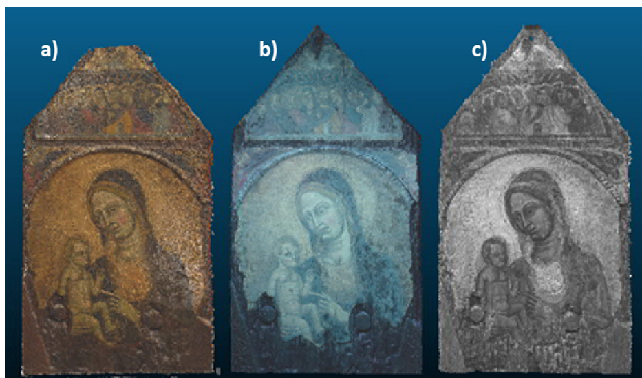
Fig. 1. 3D multispectral reconstruction of the surface of a painting. (a) RGB; (b) UV-Vis fluorescence; (c) infrared [29].
