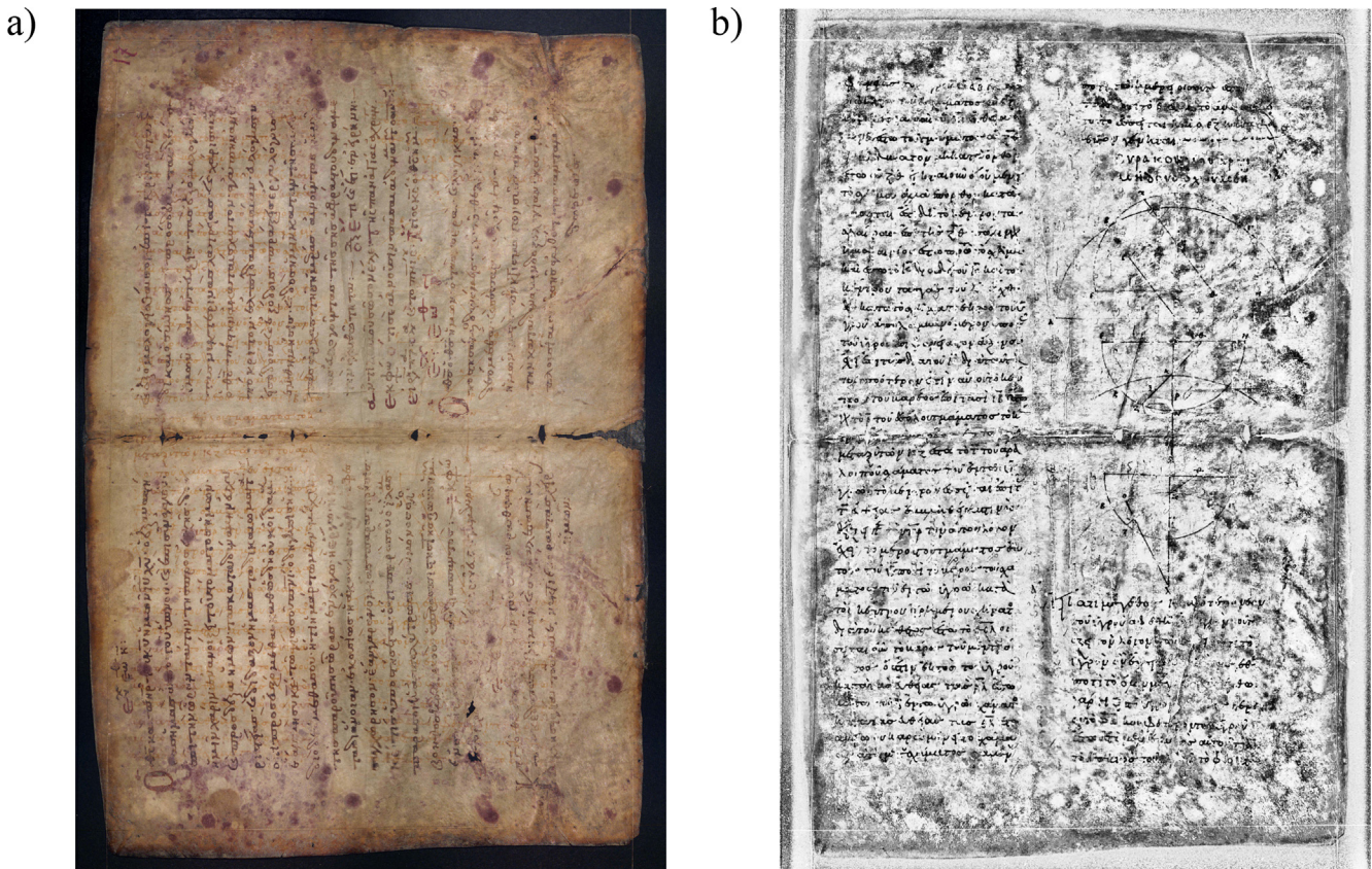
Fig. 2. Folio 16v-17r of the Archimedes palimpsest. (a) RGB image under strobe lamp illumination. (b) Second component output (contrast-enhanced) from the 2 \times 2 PCA of the red and blue colour channels, revealing the underwritten text and drawings (© The owner of the Archimedes Palimpsest, licensed for use under creative commons Attribution 3.0 Unported Access Rights. Image processing: The Institute of Information Science and Technologies, National Research Council of Italy).
