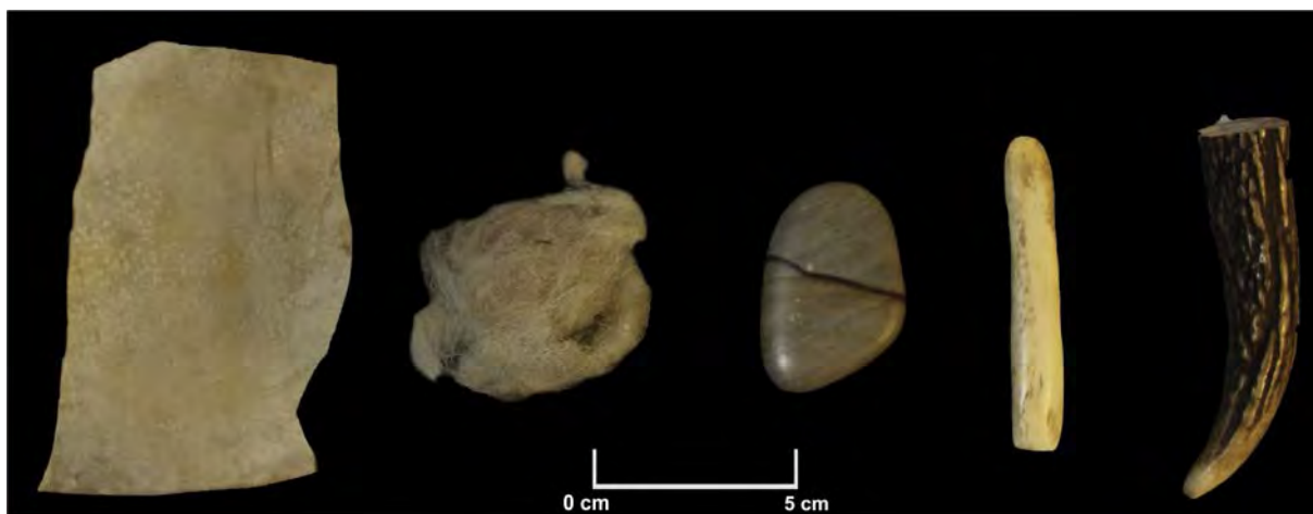
Fig. 4. Tools used for the experimental surface burnishing: leather (soft), wool (soft), cobble (hard), bone (medium hard) and antler (medium hard).
