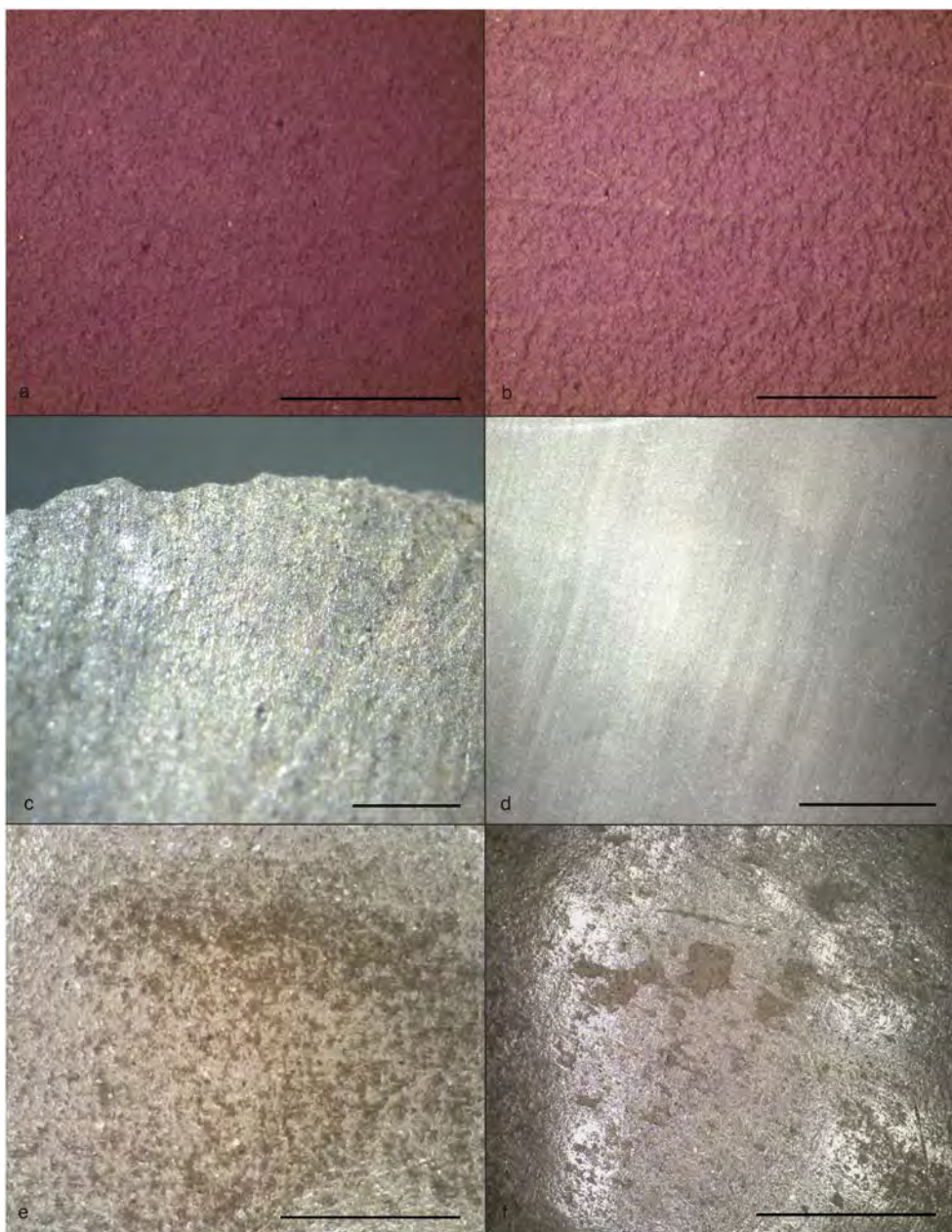
Fig. 7. Examples of experimental burnished surfaces. a: flat, dry and fine-grained clay surface before burnishing application; b: sinuous, dry and fine-grained clay surface before burnishing application; c–d: examples of a smooth burnishing with a flat topography applied at a dry stage; e–f: examples of a rough burnishing with a sinuous and rough surface (black bar is 5 mm).
