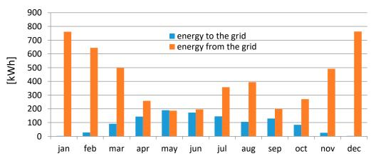
Figure 7. Monthly energy (kWh) from and to the grid, with a PV plant of 2.2 kW power.
