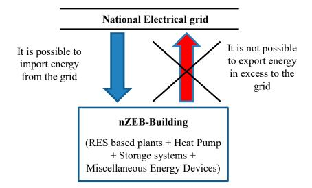
Figure 1. Logic of a net zero-energy building (nZEB). RES: renewable energy system.
