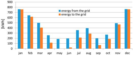
**Figure 9.** Monthly energy from the grid (PV plant of 2.2 kW, and PV plant of 2.2 kW with 6 kWh storage).
