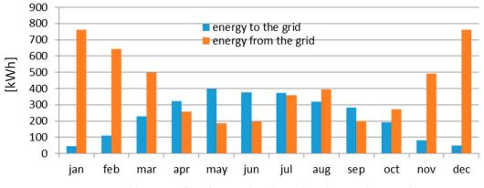
Figure 6. Monthly energy flow from and to the grid, with a 3.74 kW PV plant.
