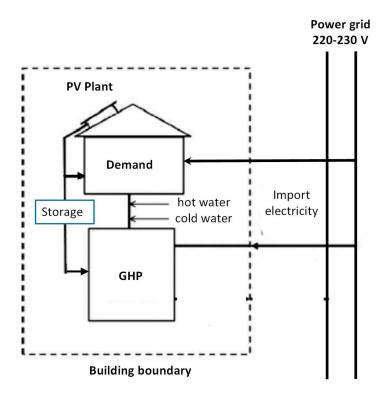
**Figure 8.** A schematic description of the plant consisting of a GHP for house heating and cooling and assisted by a PV system with a storage system (it is not possible to export energy to the grid).
