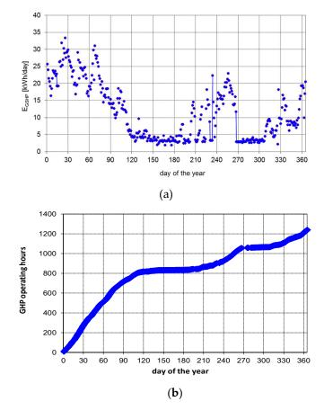
Figure 5. Daily energy consumption of the GHP in a typical year (a) and hours of operation (b).
