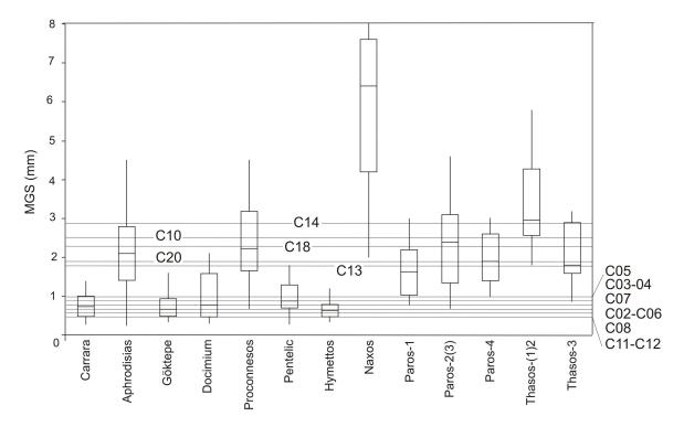
**Figure 4.** Maximum grain size (MGS) values of the analyzed marble samples compared with those of the Mediterranean area used in antiquity [21].
