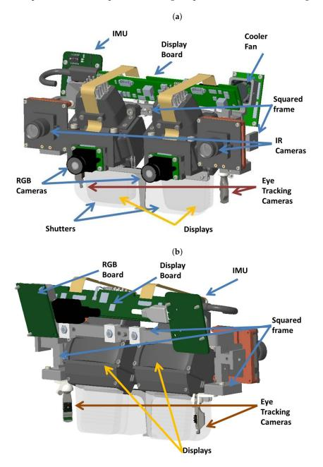
**Figure 5.** (a) Front view. (b) Back view. Layout of the opto-electronic module with its main components installed on a square frame.
