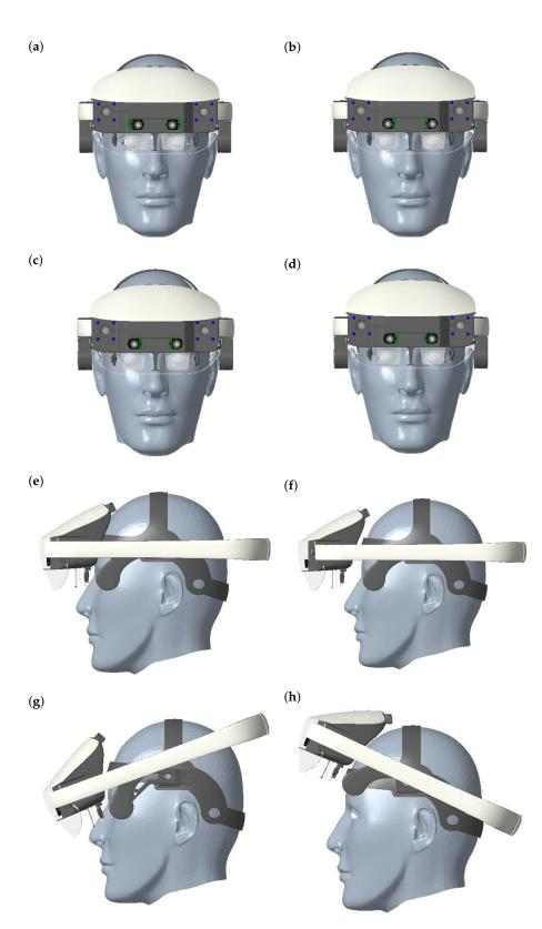
**Figure 9.** VOSTARS HMD mechanical solutions: (a) Displays with interpupillary distance set at 56 mm. (b) Displays with an interpupillary distance set at 70 mm. (c) Frontal part shifted 6 mm downward. (d) Frontal part shifted 4 mm upward. (e) Frontal part at minimum horizontal stroke. (f) Frontal part at maximum horizontal stroke. (g) Visor at maximum downward tilt for use in a surgical scenario. (h) Visor in stand-by upward condition.
