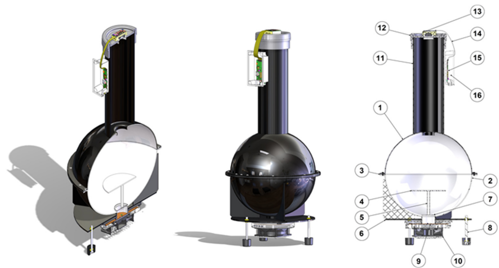
Figure 2. The rendered digital model of the proposed instrument in isometric view and main components: ①—Upper hemisphere. ②—Lower hemisphere. ③—Connection flange. ④—Deflector. ⑤—Support of the deflector. ⑥—Flange to support the sphere. ⑦—Separation glass. ⑧—Support feet. ⑨—LED illuminator. ⑩—Cooling system. ⑪—Dark tube. ⑫—Support for sensors/cameras. ⑬—Sensor/camera head. ⑭—Flat connection cable. ⑮—Sensor/camera Controlling Processing Unit (CPU). ⑯—CPU holder.
