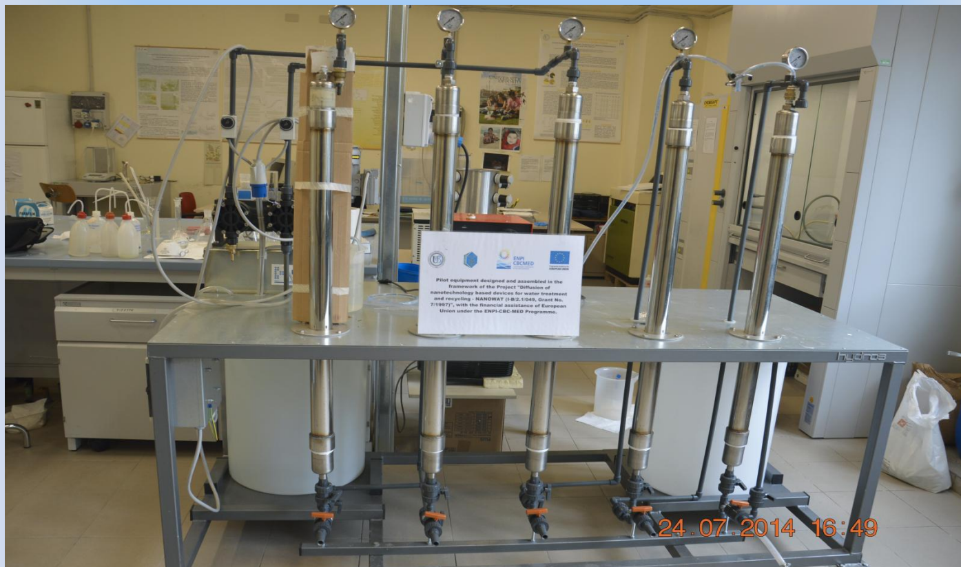
Pilot equipment designed for filtration of water containing organic and inorganic contaminants using clay-composite materials (European project NANOWAT)
