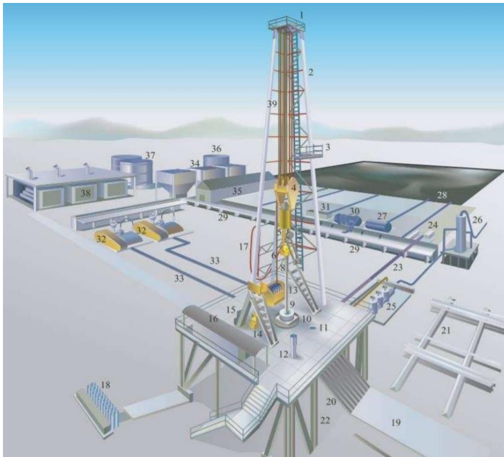
Figure 12: Drilling Ring composed by 1= fixed side; 2= derrick; 3= pontist platform; 4= mobile sides; 5= hook; 6= injection head; 7= elevators; 8= square rod or driving rod; 9= drag bushing; 10= broad bricks; 11= storage hole for the square rod; 12= storage hole for the rod to be connected; 13= winch; 14= battery weight indicator; 15= workstation of piercer; 16= booth of the perforator; 17= hose; 18= pressure accumulators; 19= rod extraction corridor; 20= slide; 21= rod shelter rack; 22= substructure; 23= mud return pipe; 24= vibrating screen; 25= surface circuit for well control; 26= gas-mud separator; 27= degassers; 28= reserve mud tank; 29= mud tanks; 30= sand removal equipment; 31= silt removal equipment; 32= mud pumps; 33= mud delivery pipe; 34= storage of materials used for sludge packaging; 35=sludge preparation cabin; 36= water tank; 37= fuel tank; 38= power generation plant; 39= cable. Translated from [61]
