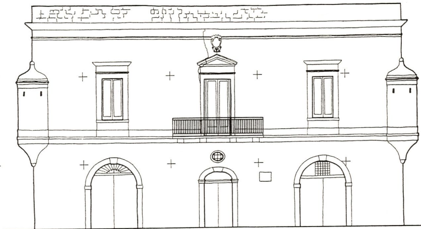
Fig. 1: Photogrammetric survey of the façade of "Masseria La Marchesa".
