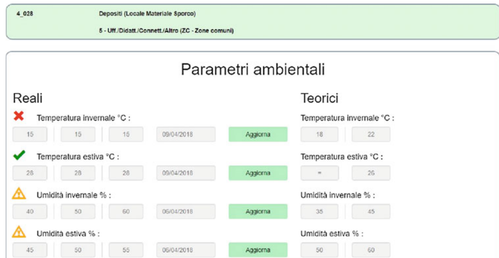
Fig. 1 Details section. Winter and summer temperatures together with winter and summer humidity are shown. Current values are displayed on the left column compared with the theoretical ones on the right side
