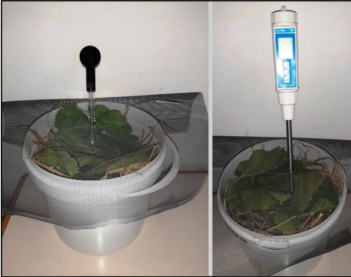
Figure 51: Application of pH and Temperature (left) and humidity (right) probe
