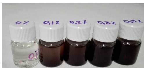
Figure 1. Photographs of the liquid phase of the acrylic bone cements' (ABCs) formulations. From left to right, the percentage of graphene oxide (GO) increases from 0 to 0.5 wt.%.
