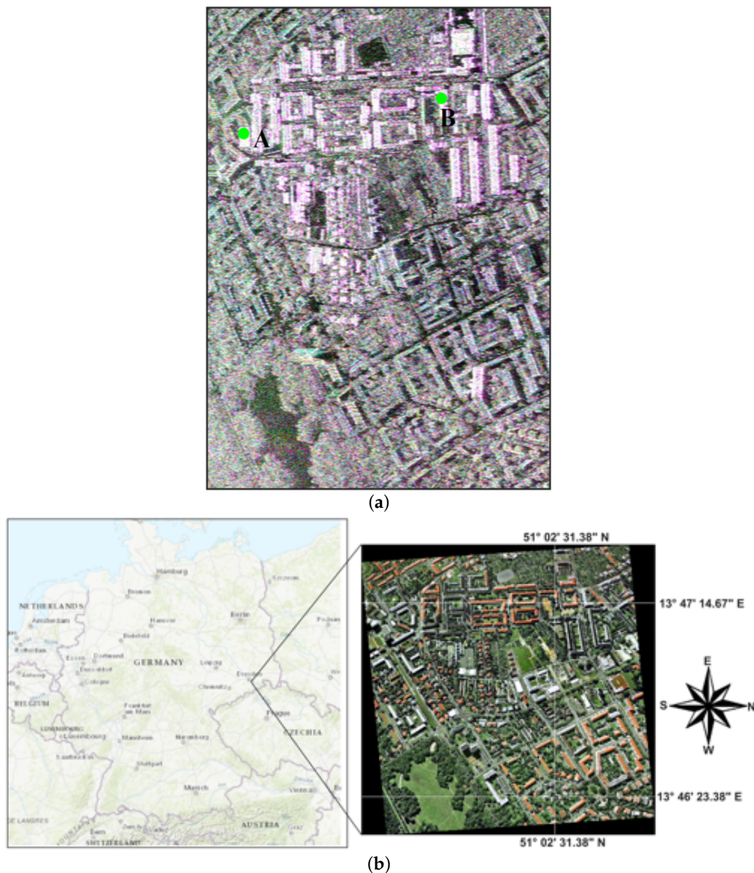
Figure 2. Information about the data set and the study area in Dresden, Germany. (a) The Pauli color composite of the polarimetric ESAR master image provided by the German Aerospace Center (DLR). (b) Location of the study area on the map of Germany (left) and the georeferenced optical image of the test area (right) (courtesy of Google Earth).
