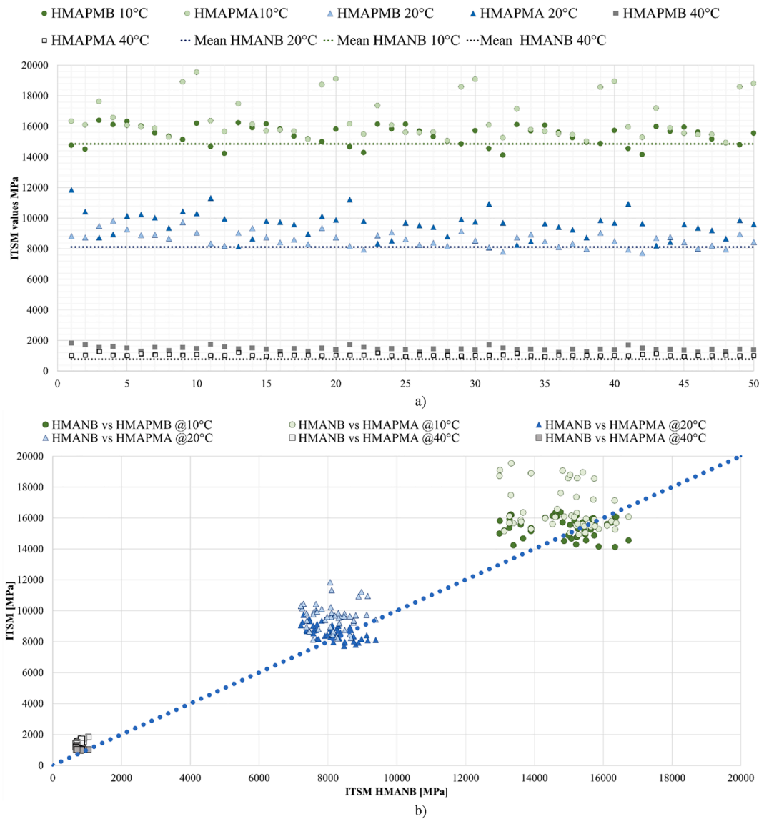
Fig. 5. ITSM evaluation a) Distribution of ITSM mean results at 10, 20 and 40 °C b) Performance diagram ITSM HMA NB vs ITSM of HMA PMB and HMA PMA .
