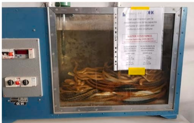
Fig. 12. Equipment for water environment at controlled humidity.
