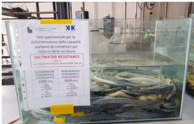
Fig. 11. Equipment for saltwater environment.
