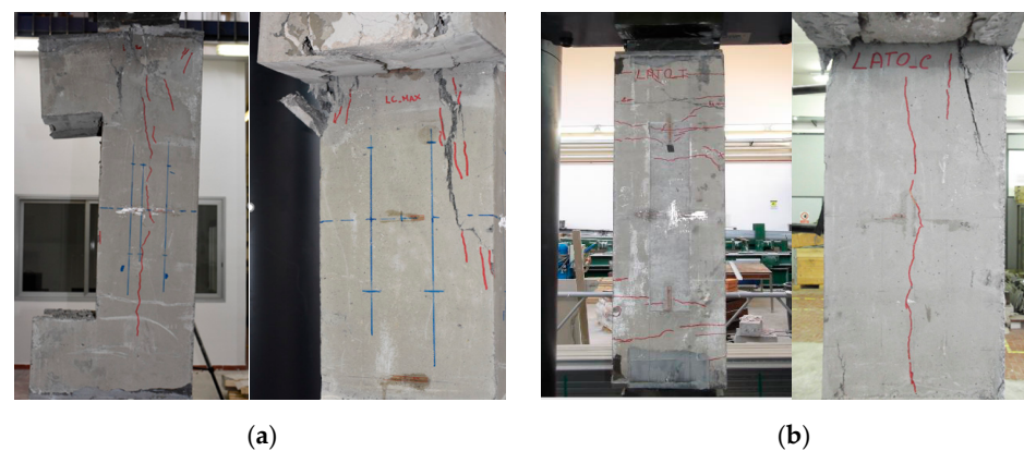
Figure 9. General views (back or lateral) and details of the final damage states for the specimen S2 (a) and S3 (b).
