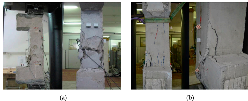
Figure 8. General views (frontal or lateral) and details of the final damage states for the specimen U1 (a) and S1 (b).
