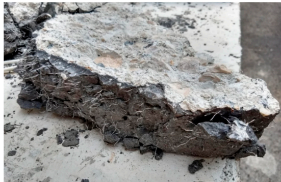
Figure 10. Detailed image of a representative interface piece removed from specimen S2.
