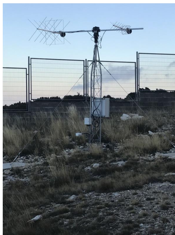
Figure 1. Montsec UHF/VHF antennas
