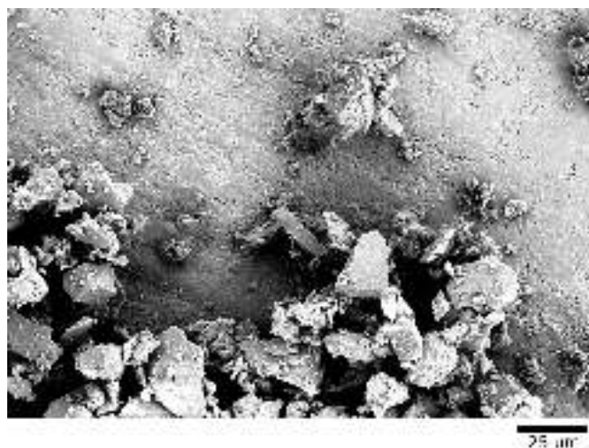
Fig. 1. Scanning electron microscope image of the basalt sample used. The mass is dominated by monomers of size \geq 20 \mu\text{m} .
