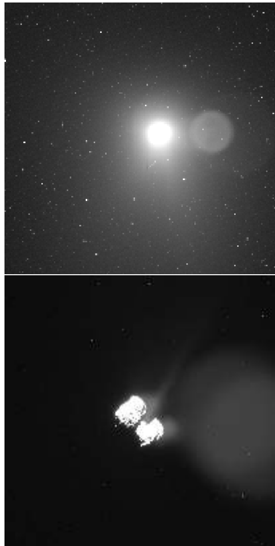
Fig. 8. Top panel: image of 67P acquired on July 25, 2014. A ghost is clearly visible on the right-hand side of the image. Bottom panel: image acquired on August 8, 2014. The ghost is in the same position as in the top panel and it is blending with the coma, creating artificial structures.
