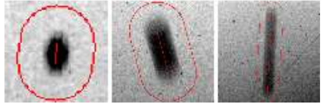
Figure 2. Example of aperture photometry with stadium shape for three different particles. The central lines mark the position of the particle and the beginning of the aperture integration. The stadium shapes mark the mask where we measured the background signal.
