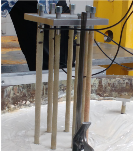
Fig. 5. Template raft for pile group installation.
