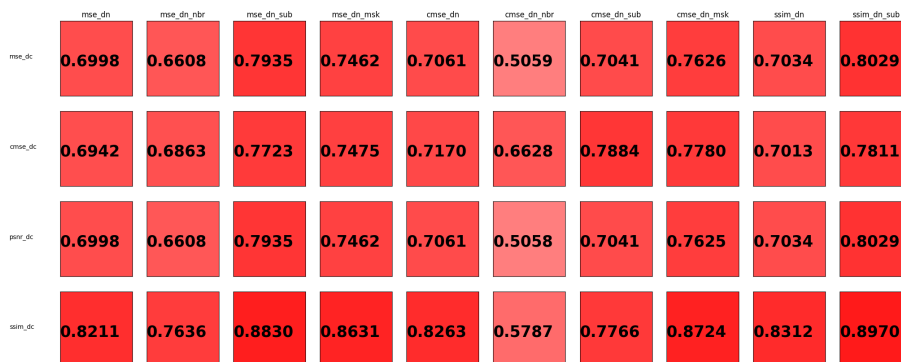
Figure 42: SRCC values of the benchmark metrics using only the images with Poisson and re-scaled Poisson noise.
