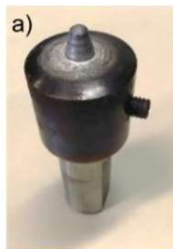
Figure 3: Tools surface after the friction stir welding processing covered with the magnesium alloy
