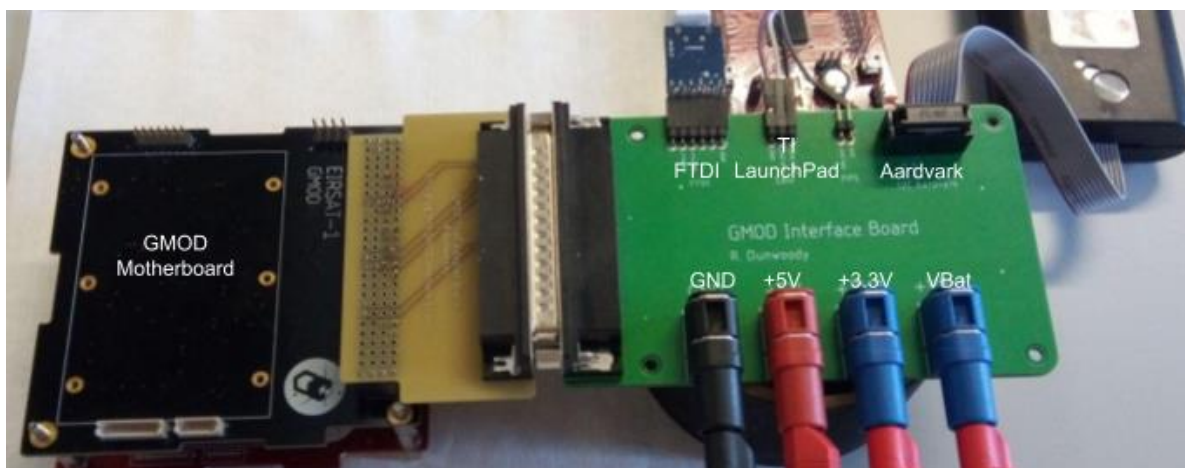
Figure 3. The hardware setup used to test GMOD firmware, including the motherboard, interface board, Total Phase Aardvark, MSP-EXP430FR5994 LaunchPad and FTDI LC234X UART module
