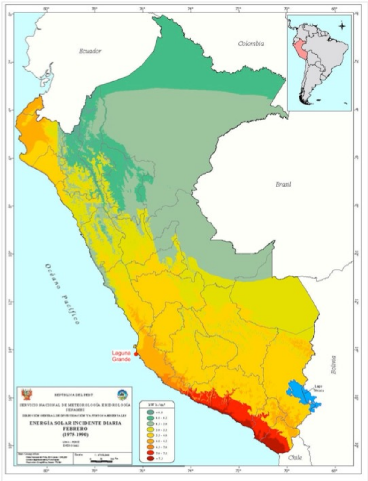
Figure 9: Solar irradiation map of Perú showing annual mean values of GHI in kWh/m 2 .day
