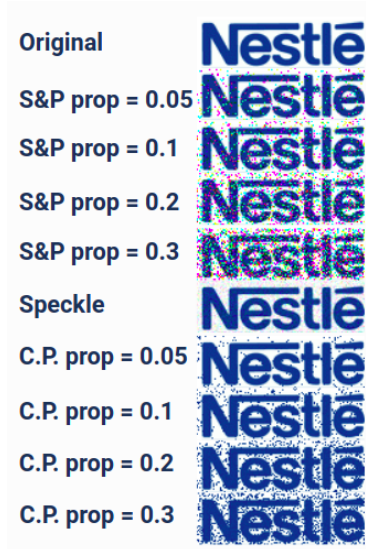
FIGURE 8.5: Salt & Pepper Noise, Speckle and Logo Color Pepper Noise. Values represent the proportion of affected pixels.
