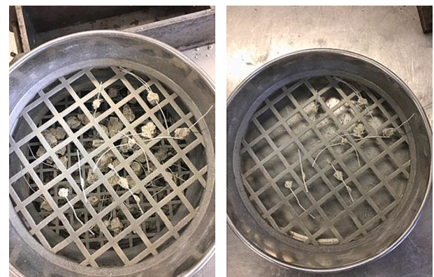
Fig. 6. Retention of RCA on the 20 mm sieve.
