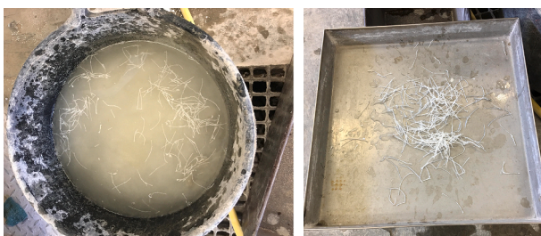
Fig. 3. Collection of recovered fibres after recycling by flotation.
