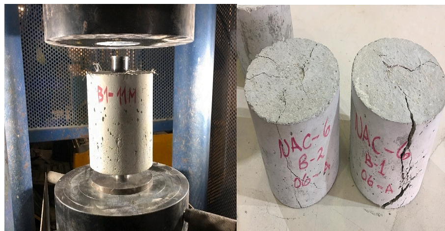
Fig. 5. Barcelona test (left) and specimens after testing (right).
