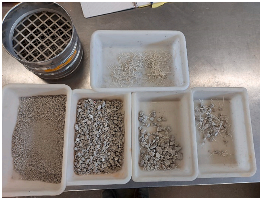
Fig. 4. Fractions of RCA obtained after sieving and used for counting embedded PP fibres. Bottom row from left to right: 0/4, 4/12, 12/20, greater than 20. Top row: recovered fibres.
