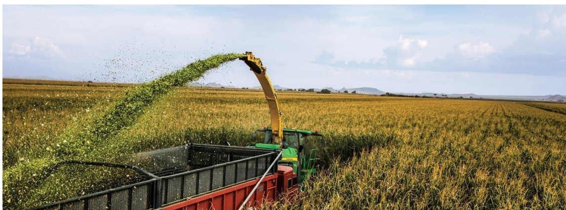
Image 10: corn chopper harvesting a corn field for silage.
