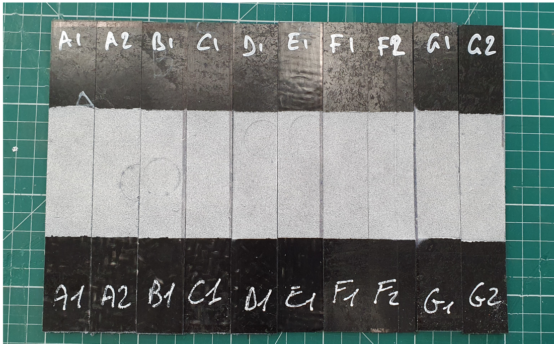
Figure 6.5: Samples painted with the speckle pattern.
