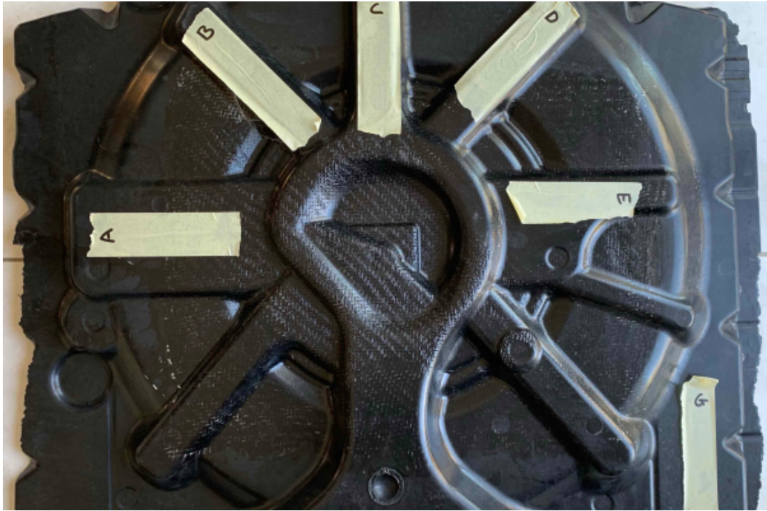
Figure 6.3: Placement of the different samples cut out from the part.
