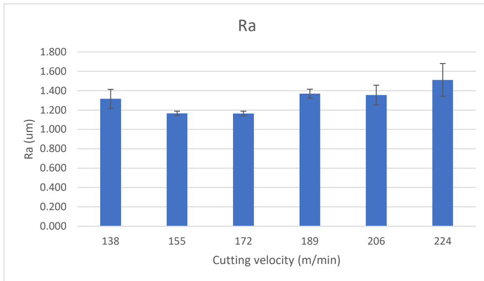
Figure 18: the arithmetical mean deviation of the roughness profile (Ra) depending on the cutting velocity
