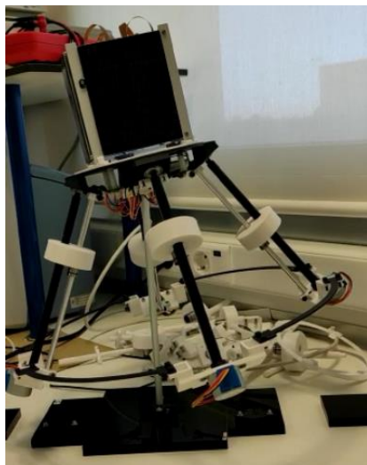
Figure 7. Testbed with automatic reposition of the center of gravity.
