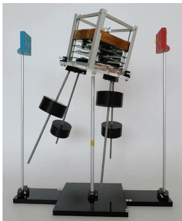
Figure 4. Three-axis magnetic-controlled ESAT and testbed prototype.
