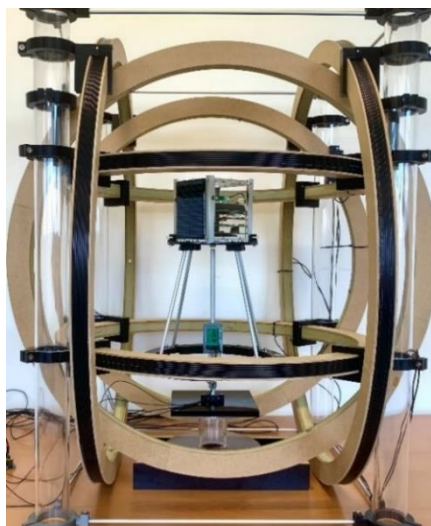
Figure 8. ESAT inside the Earth magnetic field simulator on the one-axis turntable.
