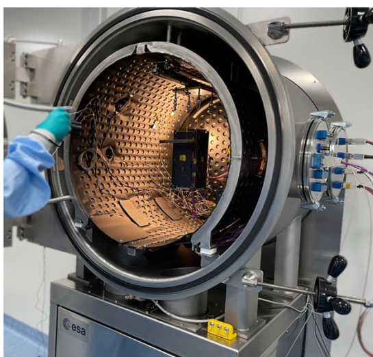
Figure 5. EQM integrated in the TVAC chamber.
