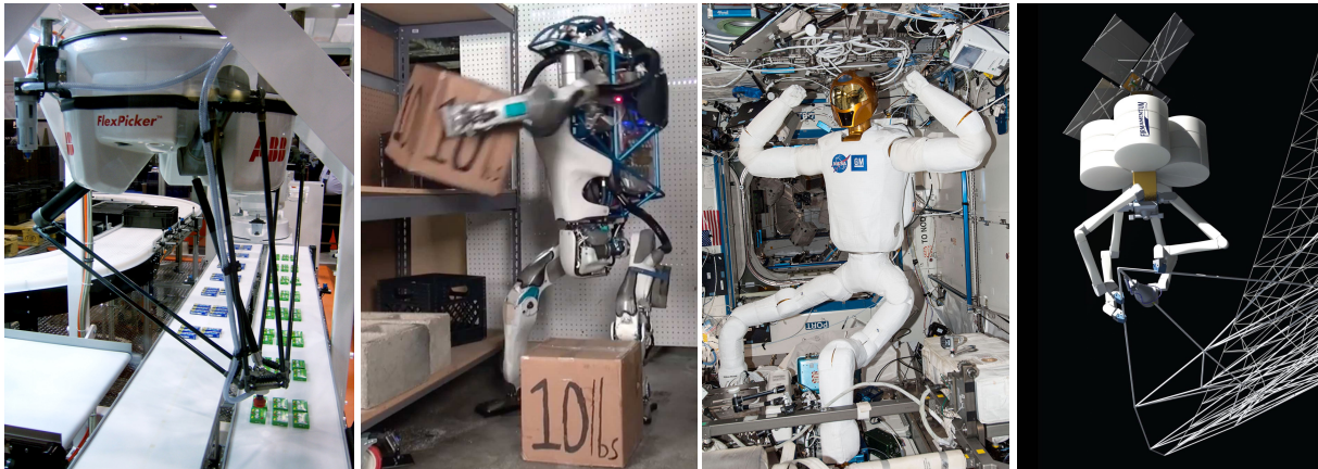
Figure 1.2: Example systems involving closed kinematic chains. The chains may be intrinsic to the robot structure, as in parallel robots (left picture), or they may result from manipulation constraints during a task, as in multi-limbed systems transporting an object, or keeping their feet attached to the environment (right pictures). From left to right: A Delta parallel robot [3], the Atlas robot from Boston Dynamics lifting a heavy load[4], the Robonaut 2 robot with two legs clamped to the International Space Station [5], and SpiderFab Bot, a conceptual design for self-fabricating space systems [6]. Pictures courtesy of ABB, Boston Dynamics, NASA, and Tethers Unlimited, Inc, respectively.
