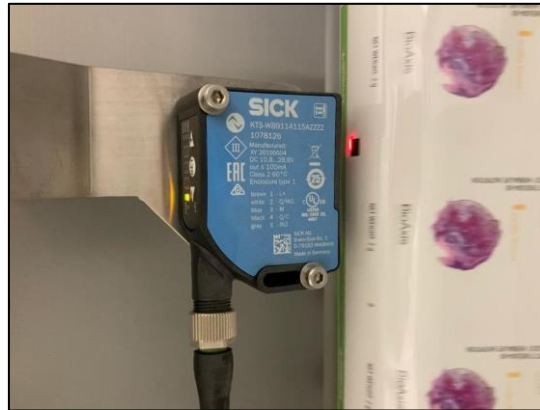
Figure 42. External sensor reading a contrast mark
