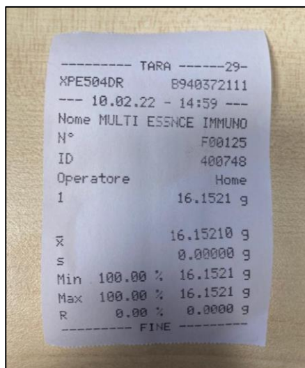
Figure 41. 10 sticks weighed at once (left) and its corresponding printout with the total weight (right)
