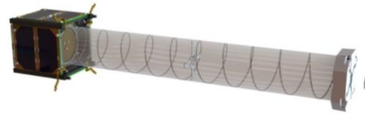
Figure 2 - NADS in deployed configuration
