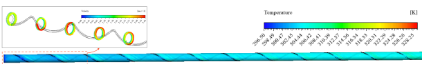
Figure 5: Pinhole wall temperature contour and velocities distribution in transversal cross-sections for Stage 3 case.
