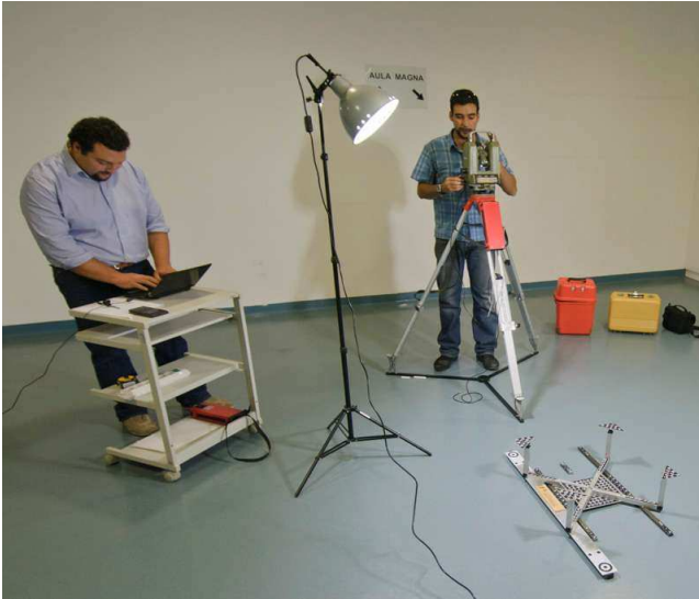
Figure 3. Calibration frame and scale bar (up) arranged for laboratory measurement (down).
