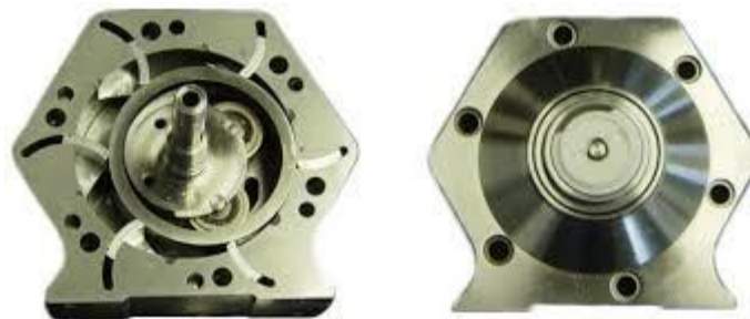
Fig. 14: 6-chamber Di Pietro engine. Left: front view. Right: rear view.
