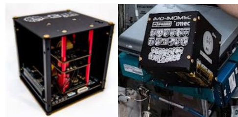
Figure 4: left) Finished QUBE without side panels. right) the QUBE onboard the ISS during installation by Thomas Pesquet.
