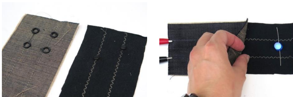
Figure 19. 3D Printed conductive snap buttons on fabric. (Source: [17])
