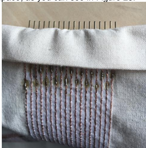
Figure 28. Row of male header pins embedded onto a textile (Source: [26])
