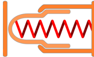
Figure 20. Cross section of Pogo Pin in contact with a pad. (Source: Google)
