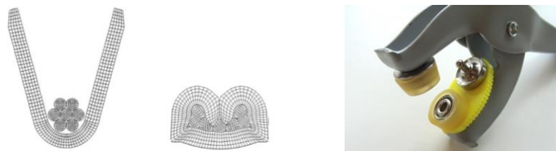
Figure 16. Open crimp barrel and wire before and after crimping (left) [15].
