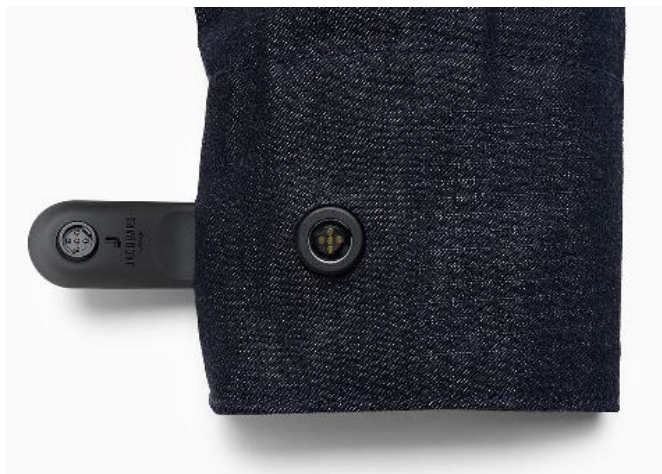
Figure 4. Bluetooth device attached as a cufflink (Source: textiletoday.com).
