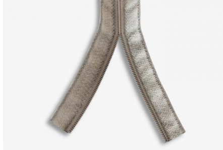
Figure 23. Conductive zipper (Source: [22])
