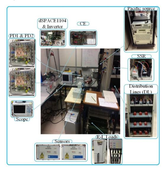
Figure 9. Complete laboratory setup.
