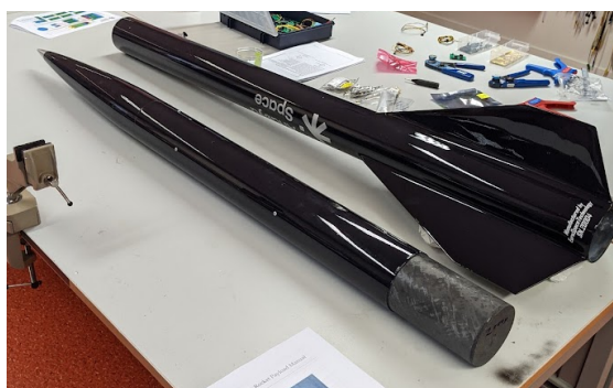
Figure 1. Rear airframe (above) and avionics tube (AT) with nose cone installed (below).
