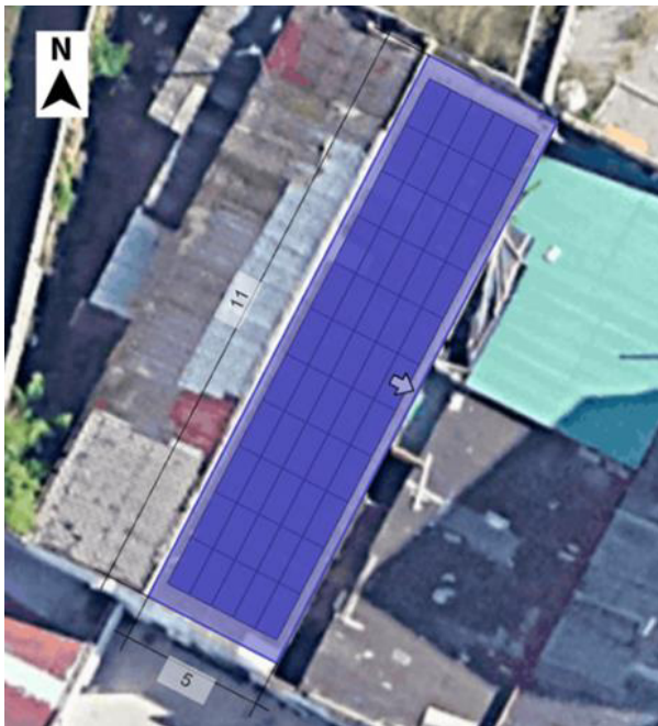
Figure 4-8: PV installation designed with K2Base
