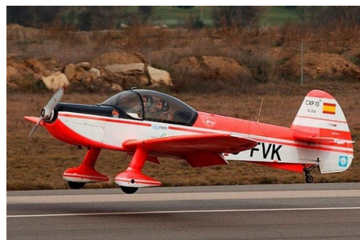
Figure 1. Mudry CAP10B aerobatic aircraft used for educational parabolic flight campaigns. (Credit: Barcelona-Sabadell Aviation Club)
