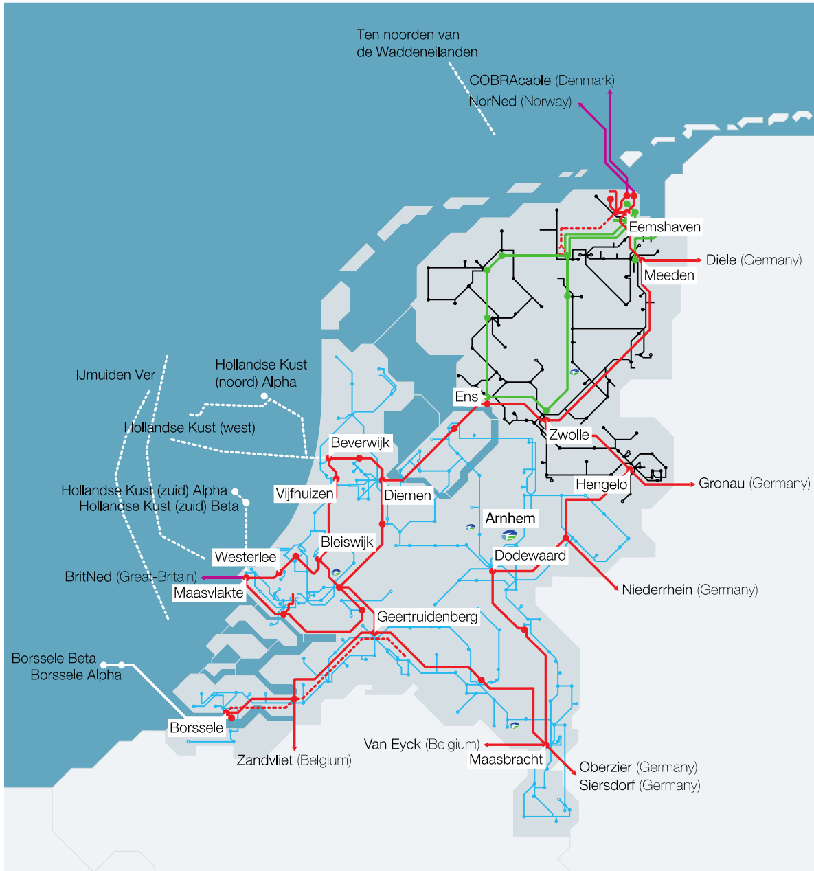
Figure 9: Map of the TenneT's high voltage physical grid in the Netherlands – red: 380kV, green: 220kV, blue: 150kV, black: 110kV [24]
