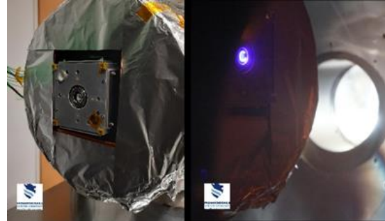
Figure 3: Thermal vacuum testing of CLIMB's thermal model with ENPULSION's NANO thruster.
