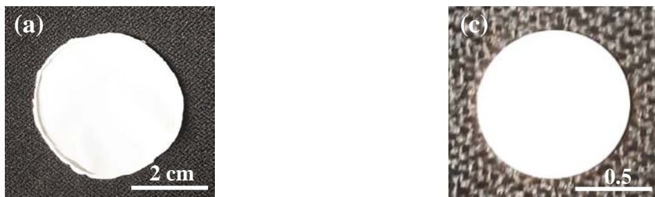
Figure 3. Solvent casting films obtained from PBS/Poly(PA-LO) 70:30 (a), PBS/Poly(PA-LO) 50:50 (b) and a pressed tablet of pure Poly(PA-LO) (c)
