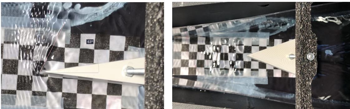
Figure 12. Left) Example of an oblique hydraulic jump; Right) Example of a detached shock wave
