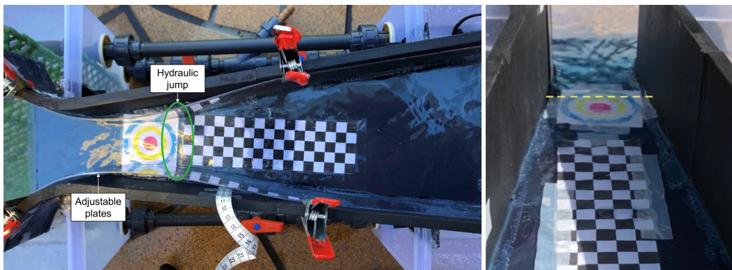
Figure 10. Examples of a hydraulic jump and the adjustable plates
