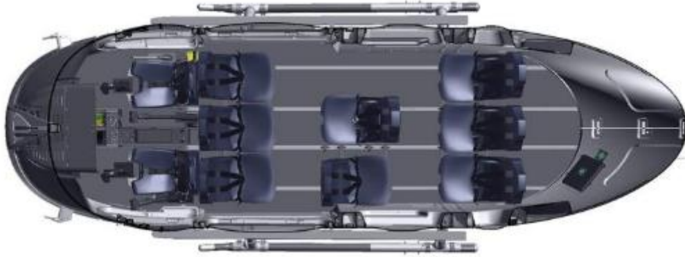
Fig. A.2.8. Eight seats for passenger transport configuration of the Airbus H145 [44]
