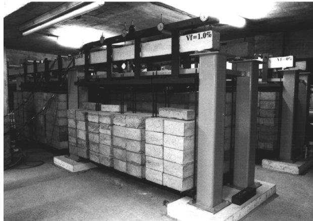
Fig. 8. Experimental setup for testing FRC beams (authorized reprint from [98]).
